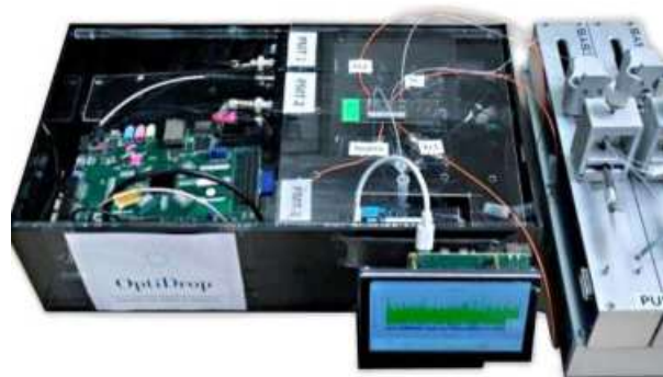
OptiDrop is developed using a proprietary microfluidic chip with integrated optical fibres photomultiplier tubes and a pulse counter.
