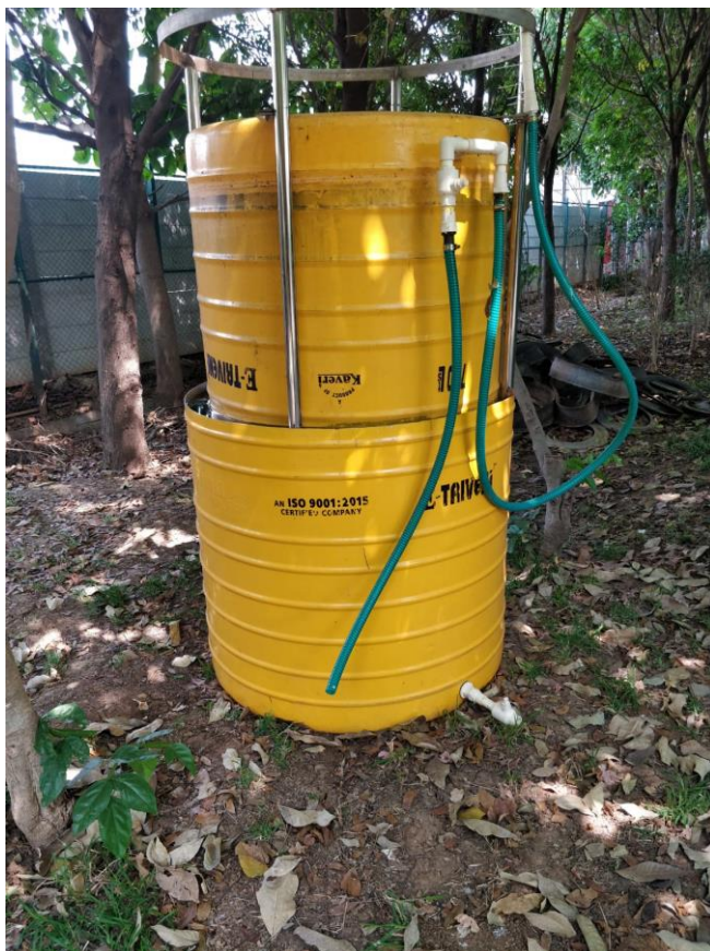
Gas collection unit filled with biogas. (During the second training, the feed from first week had digested)
