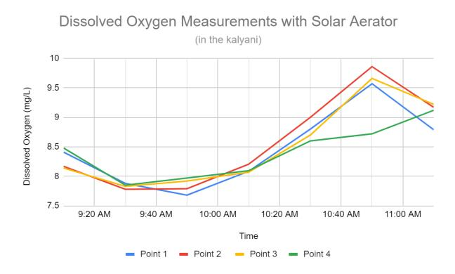
Graph 3: DO Measurements with Solar Aerator
